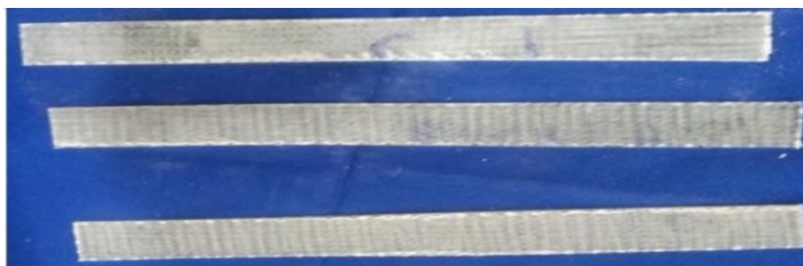
Figure 4 Shows the samples preparation 3mm thickness after phenol coat
