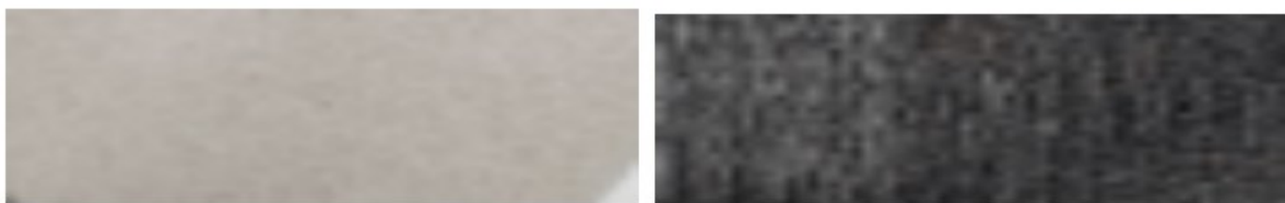
Figure 2: Carbon fibre laminate with and without phenol coat
