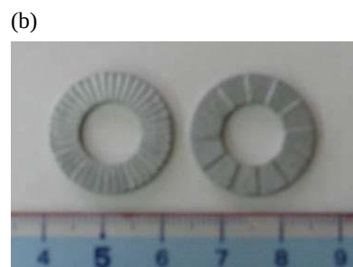
Fig. 8. Test specimens with both-sides edge cracks, (a) The case of a normal and bolted stop-hole, (b) Comparison of the effect of friction of washers A and B on crack initiation, (c) Specimen for testing the effect of crack arresters
