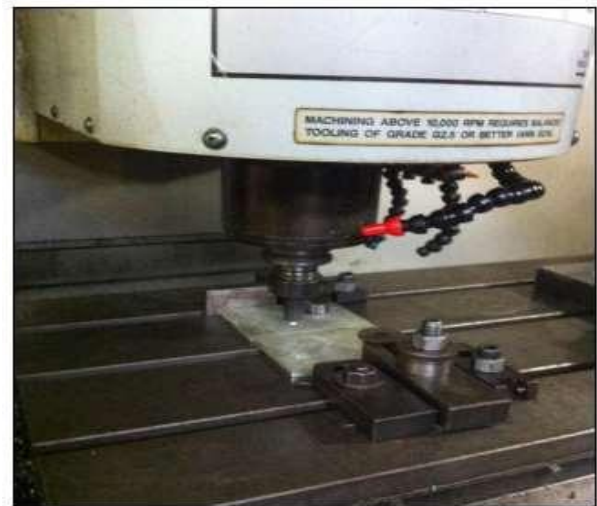
Figure 2. Starting Stage of FSW Process
