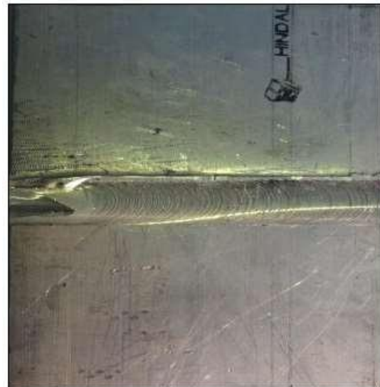
Figure 3. Welded Specimen at 1100 rpm, 70mm/min
