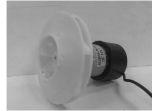
Fig. 3 Centrifugal fan connected to the DC motor
