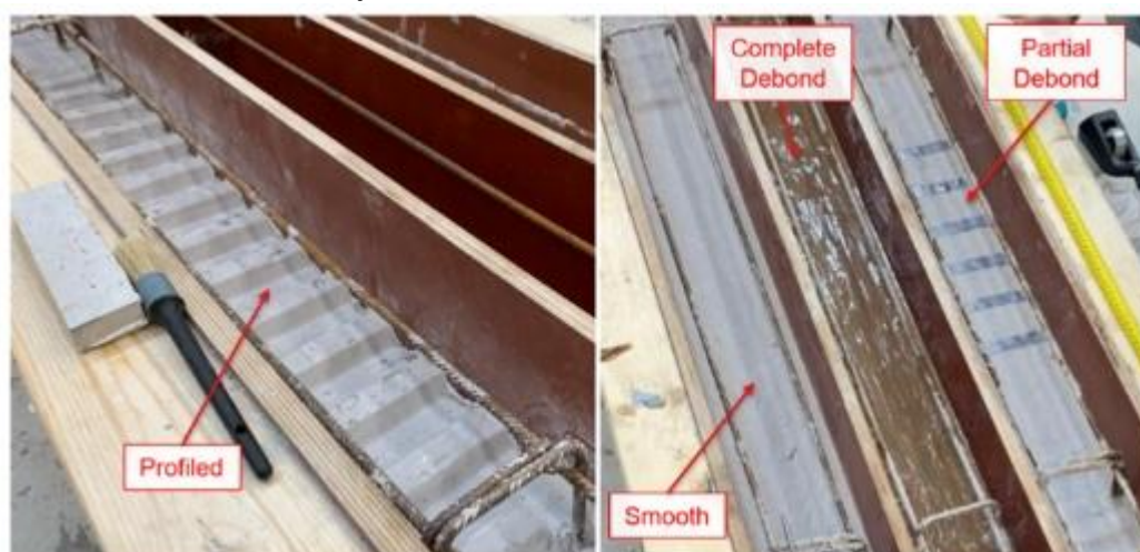
Fig. 3. Interface preparation of the hybrid beams before casting the concrete top layer.
