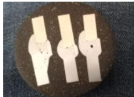
Figure:2 Sample preparation for micro structure, hardness, tensile
