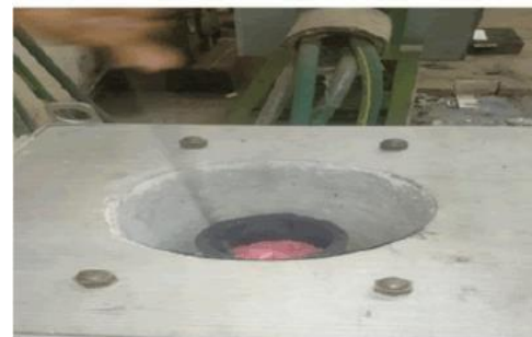
Figure 1: Stir Casting On Pit Furnace
